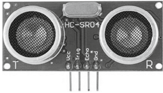
Fig. 2.1 An image of ultrasonic sensor (HC-SR04)
